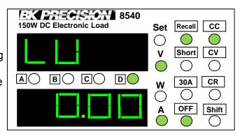
Programmable Range: 0.00 – 60.00 Use the ■ keys to change cursor position shown by the LED light next to either A, B, C, or D (These four denotes cursor position, with A selecting the most significant figure and D the least significant figure.
